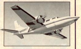
**1982.** On November 30, Piper introduces the Aerostar 700P, an improved version of the 601P with turbocharged, intercooled 350-hp Lycoming TIO-540-U2A engines.
